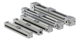
JBO linear units offer a large product portfolio in flat design with toothed belt or ball screw drive. These units are available up to a length of 6m and can be equipped with one or two carriages. Due to a lifetime grease lubrication the units are very low maintenance. The different axis systems can be combined to a portal with X-, Y- and Z-axis.
